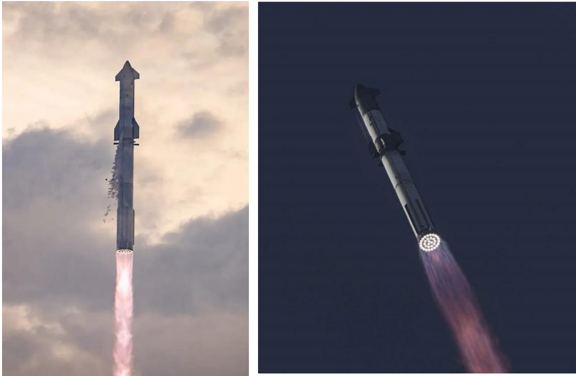
Figure 7-8 STARSHIP AT SEA-LEVEL (LEFT) AND AT ALTITUDE. NOTE THE EXHAUST PLUME IS NARROW AT SEA LEVEL, INDEED IT NECKS DOWN A BIT, INDICATING OVEREXPANDED EXHAUST. AS THE STARSHIP GAINS ALTITUDE THE PRESSURE DECREASES AND THE EXHAUST STARTS SPREADING OUT- THE EXHAUST IS NOW UNDEREXPANDED.
